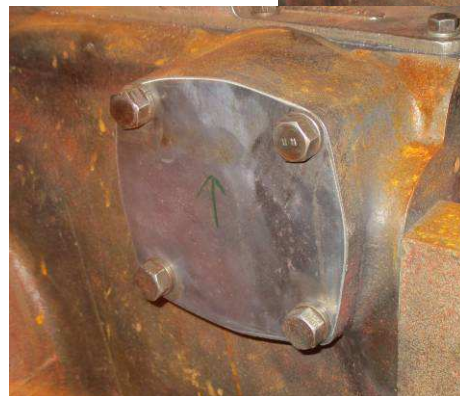
Finished covers. PTO delete above and belt pulley delete to the left. There is nothing like holding on a sheet metal cover with 1/2"-13 bolts!
