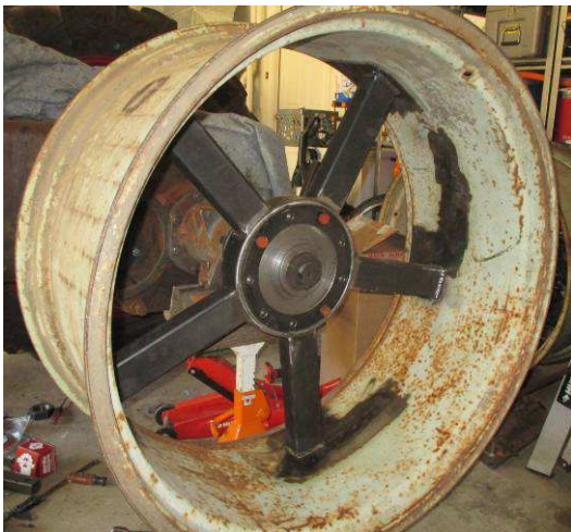
Rim welded and fitted to the MH 101
